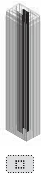
Braced core Aon Center 707 Wilshire Blvd. Completed: 1973
