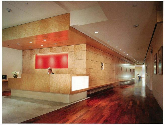
Lighting defines architectural planes in the reception area for Warner Home Video (left and below). A flatscreen monitor framed by frosted glass is inset into a red-painted wall. Cold-cathode fixtures outline the top and bottom edges of the red wall. As a visual pivot point in a corridor, a structural column is wrapped with fluorescent strip lights behind translucent panels (opposite, top). Backlit horizontal panels enhance corridors (opposite, bottom).
